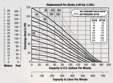
NOTE: Performance based on the following: elastomeric fitted pump, flooded suction, water at ambient conditions. The use of other materials and varying hydraulic conditions may result in deviations in excess
