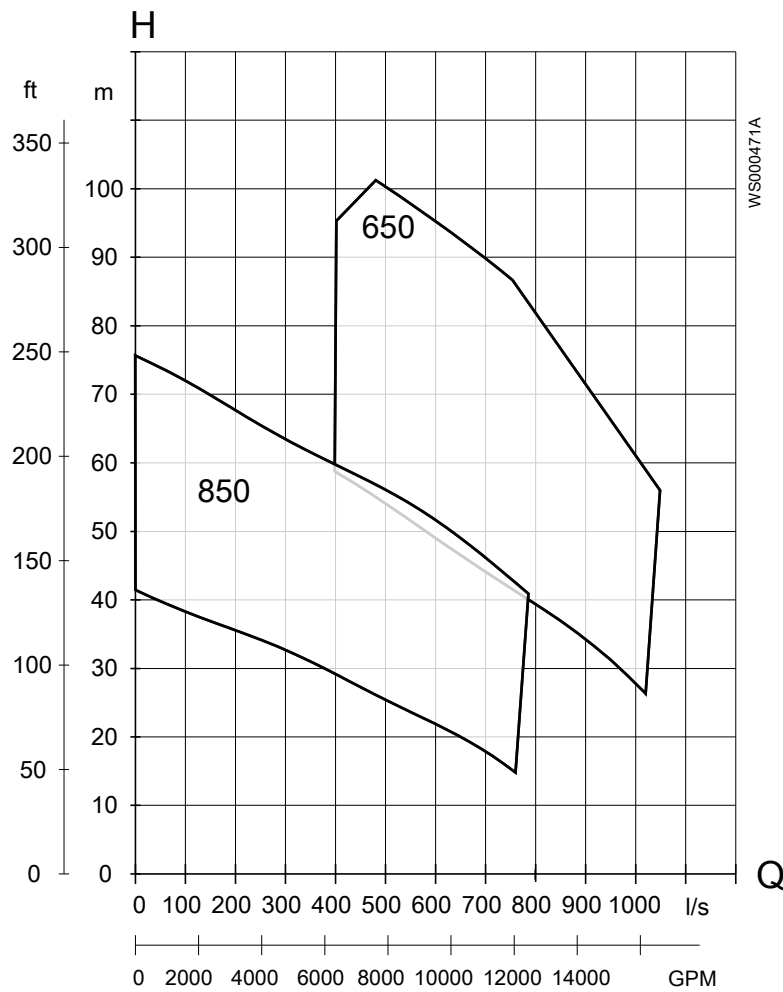
Figure 80: C3351, 60 Hz, low voltage
