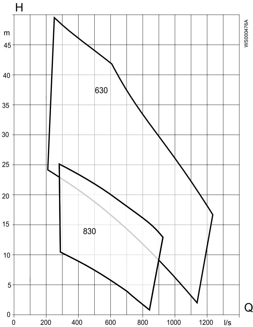
Figure 61: C3400, 50 Hz, medium voltage
